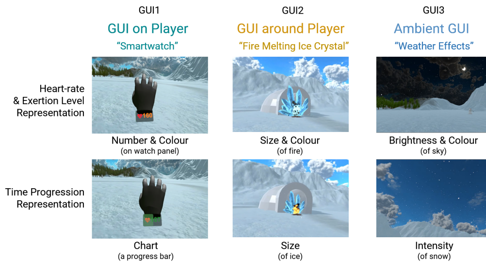
Fig. 2. Data representation in each of the GUIs, highlighting how each GUI represents heart-rate data and progression towards an exercise time goal.
